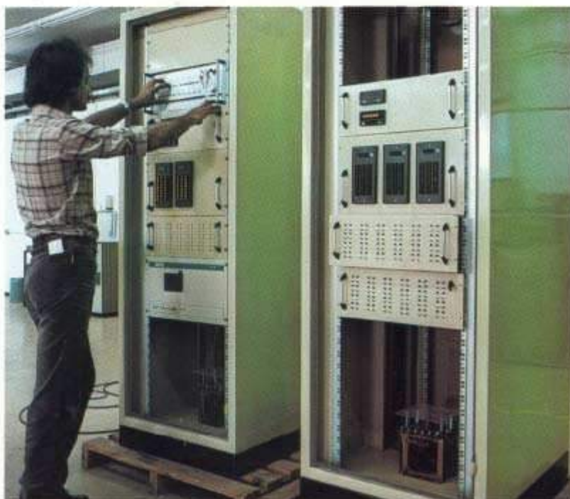
Brewer's process control system undergoing production tests
